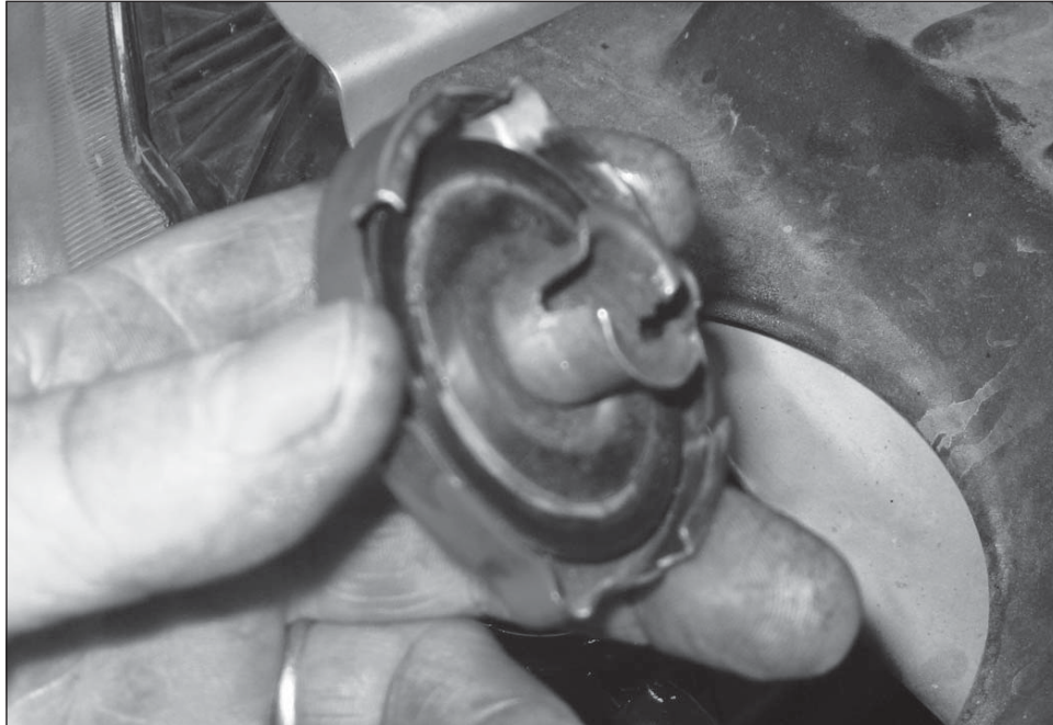
Figure 10: This is a modified radiator cap I painted red (so I remember not to leave it on) with its lower seal removed. With this cap installed, fill the cooling system as full as you can, then start the engine. The cooling system can expel air and draw in coolant as needed from the overflow bottle (you just have to watch the level in the bottle). This method builds no pressure on the system and prevents coolant surges that tend to flood the service bay and wet the serpentine belt and pulleys. Remove this cap and replace it with a good or new cap when the coolant is warm and the system is full.
