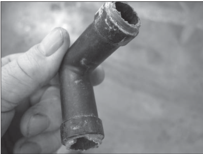
Figure 3: Coolant passes through the tensioner (as seen in Figure 1) by way of a couple of plastic elbows that routinely fail while the tensioner is still good.
