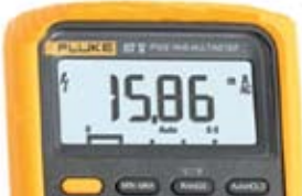
Digital multimeter incorporating a bar graph
