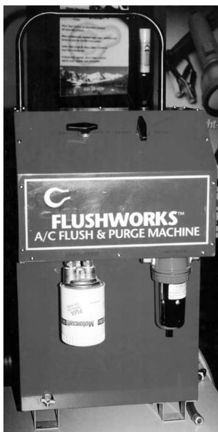
Ford approved Flushing machine, with specific terpene solvent, is used in closed loop circuits through hoses, lines, heat exchangers, followed by a shop air purge so virtually no solvent remains in any component.
