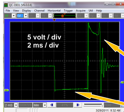
New Coil Primary ignitions coil pattern (negative side of coil)
